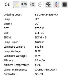
Input Voltage: 220–240Vac 50/60Hz
