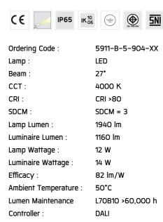
Input Voltage: 220–240Vac 50/60Hz
