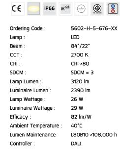
Input Voltage: 220-240Vac 50/60Hz
