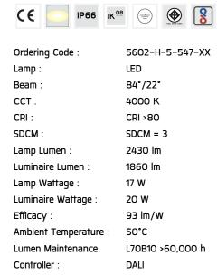
Input Voltage: 220-240Vac 50/60Hz
