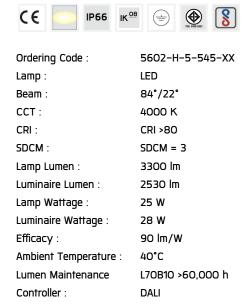
Input Voltage: 220-240Vac 50/60Hz
