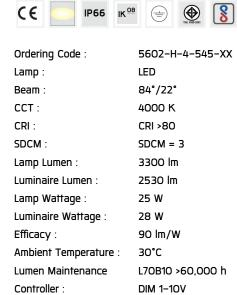
Input Voltage : 220–240Vac 50/60Hz
