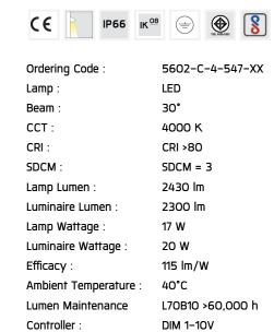
Input Voltage: 220-240Vac 50/60Hz
