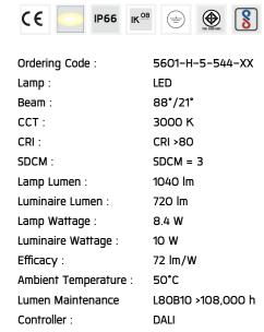
Input Voltage: 220-240Vac 50/60Hz
