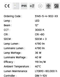
Input Voltage: 220–240Vac 50/60Hz
