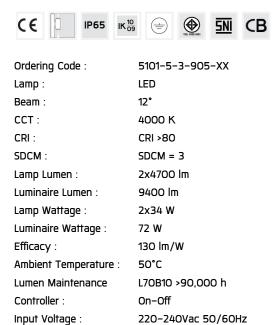
Ordering code guide XXXX-X-X-XXX-XX À Product Code Reflector C D Electrical Component Lamp Color
