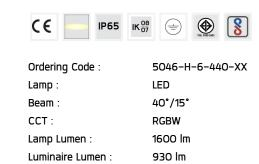
Lamp Wattage: 22 W Luminaire Wattage: 27 W Efficacy: 34 lm/W Ambient Temperature: 50°C Controller:
