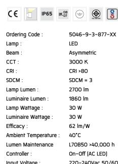
Input Voltage: 220-240Vac 50/60Hz
