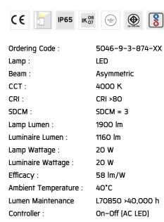
Input Voltage: 220-240Vac 50/60Hz
