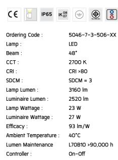
Input Voltage: 220–240Vac 50/60Hz
