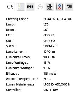
Input Voltage: 220–240Vac 50/60Hz
