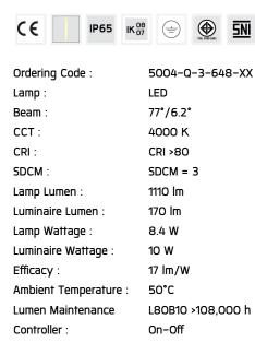
Input Voltage: 220-240Vac 50/60Hz
