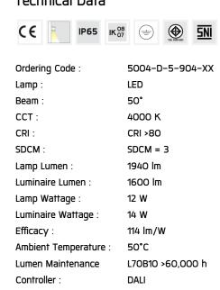
Input Voltage: 220-240Vac 50/60Hz
