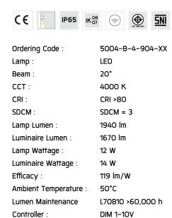
Input Voltage : 220–240Vac 50/60Hz
