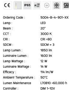
Input Voltage: 220-240Vac 50/60Hz
