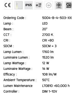
Input Voltage: 220-240Vac 50/60Hz
