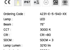
Luminaire Lumen :2380 lmLamp Wattage :20 WLuminaire Wattage :25 WEfficacy :95 lm/WAmbient Temperature :50°C
