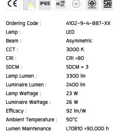
Lumen Maintenance L70B10 >90,000 h Controller: DIM 1-10V
