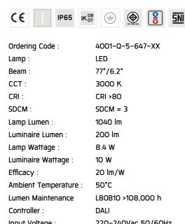
Input Voltage: 220-240Vac 50/60Hz
