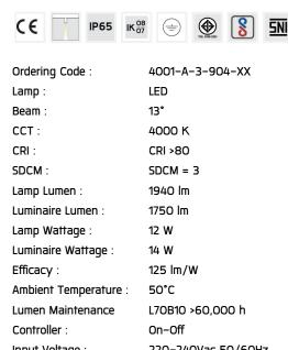
Input Voltage: 220-240Vac 50/60Hz
