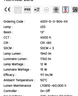
Input Voltage: 220-240Vac 50/60Hz
