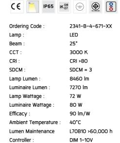
Input Voltage : 220–240Vac 50/60Hz
