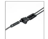
Ordering Code: AUN-CON-0010-00 IP68 Water Tight Connecting Device with Distribution block, 3 pole, 1 input, 2 outputs, Cable Diameter 5.0 - 9.5mm.
