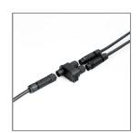
Ordering Code: AUN-CON-0010-00 IP68 Water Tight Connecting Device with Distribution block, 3 pole, 1 input, 2 outputs, Cable Diameter 5.0 - 9.5mm.
