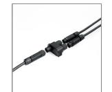
Ordering Code: AUN-CON-O010-00 IP68 Water Tight Connecting Device with Distribution block, 3 pole, 1 input, 2 outputs, Cable Diameter 5.0 – 9.5mm.
